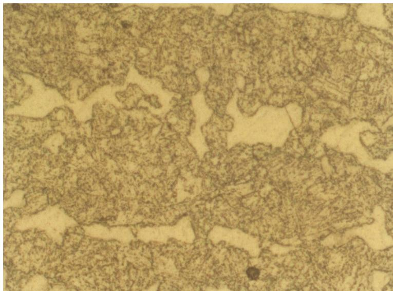
**Figure 12.** The development of metallic carbides in the case of spray coating metallization with oxy torch without ultrasound activation, in the close vicinity of the demarcation line, in the base material: base material: X30NiMoVCr11- Application material: STELLITE 12 AWS,W; Treatment: Nital 2%, Magnification 100X[6]
