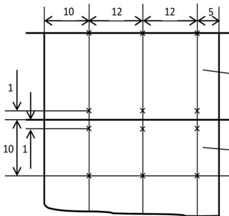
**Figure 8.** Scheme for determining the HRA hardness, as per ASME WS - 001711, on a sample taken from the reconditioned part
