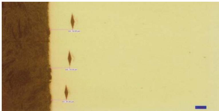
**Figure 11.** Measurement of the hardness in the close vicinity of the demarcation line in the application material
