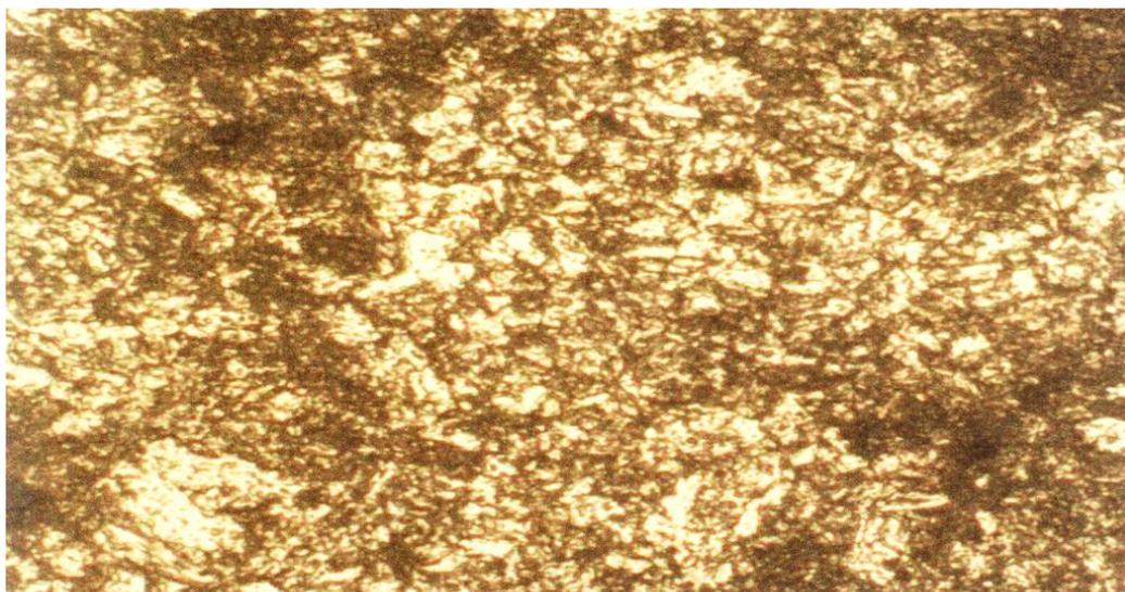
**Figure 3.** Structure of the base material adjacent to the demarcation line for the sample obtained by ultrasound field metallization: treatment: Nital solution 2%; magnification 500X
