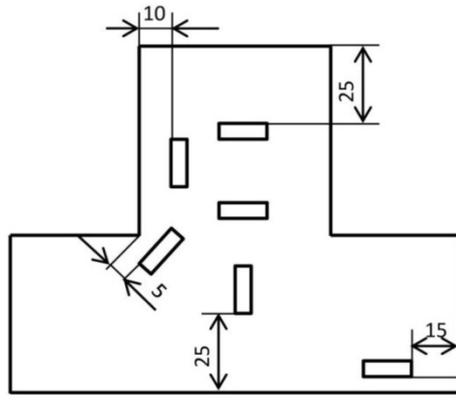
**Figure 6.** Place of sampling for traction testing
