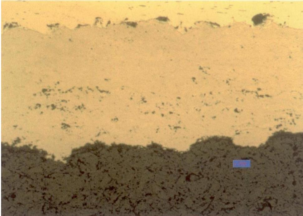
**Figure 4.** Adhesion of the first layer of application material and of the second layer, in the case of spray coating metallization without ultrasound activation: Nital; magnification 200X; base material: X30NiMoVCr11; application material: TP 4000[6].
