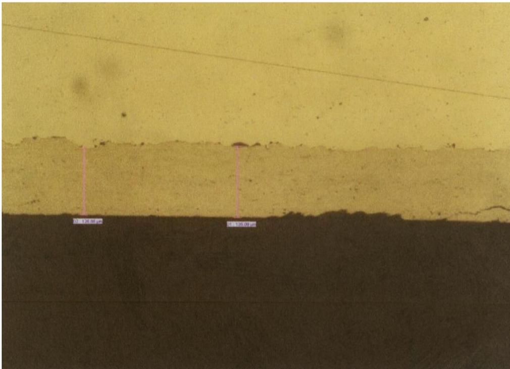
**Figure 5.** Adhesion of the first layer of application material and of the second layer, in the case of spray coating metallization with ultrasound activation: Nital 2%; magnification 200X; base material: X30NiMoVCr11; application material: TP 4000
