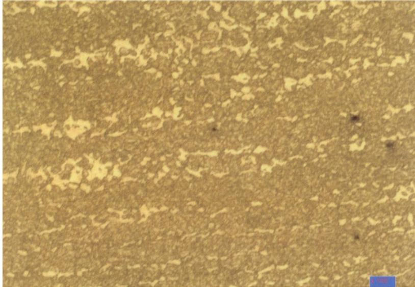
**Figure 13.** The development of metallic carbides in the case of spray coating metallization with oxy torch and powder with ultrasound activation of the part to be reconditioned, in the close vicinity of the demarcation line, in the base material: base material: X30NiMoVCr11- Application material: STELLITE 12 AWS,W; Treatment: Nital 2%, Magnification 100X[6]
