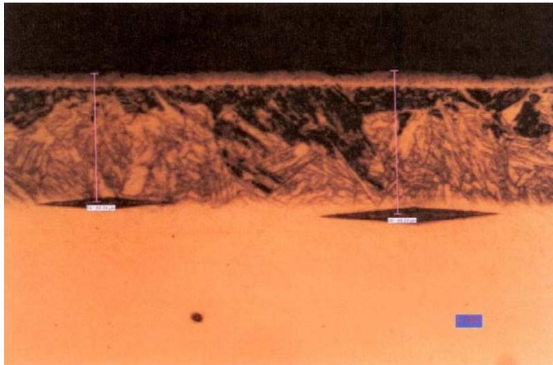
**Figure 10.** Measurement of the hardness in the close vicinity of the demarcation line in the base material
