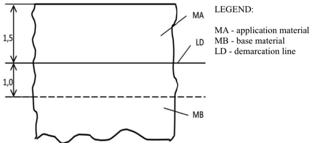
Figure 1. Scheme of measuring the chemical composition around the demarcation line
