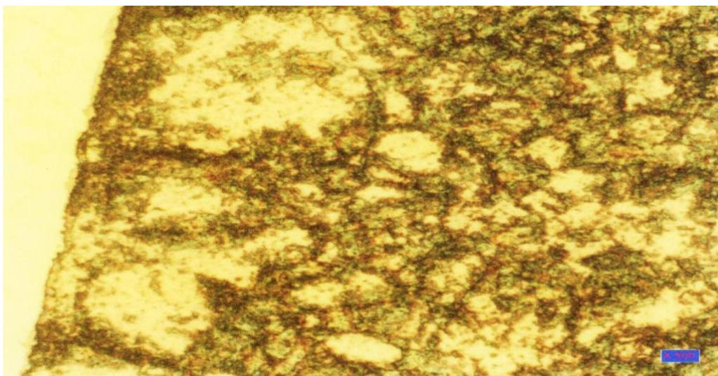
**Figure 2.** Structure of the base material, adjacent to the demarcation line in the metallized sample without ultrasound activation: treatment: Nital solution 2%; magnification 500X
