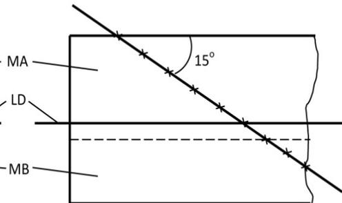
**Figure 9.** Scheme for determining the HV10 hardness, as per ISO 15614 - 7, on a sample taken from the reconditioned part
